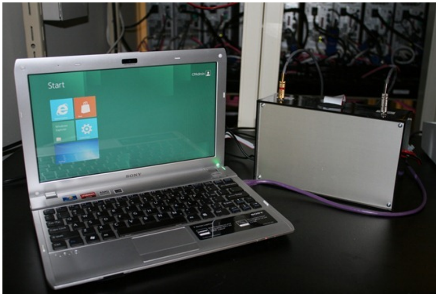
Reference platform instrumented for DC power supply and measurement
