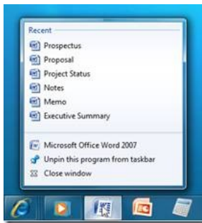
Fig 5. Jump List: Right-clicking on Word gives quick access to recently used documents
